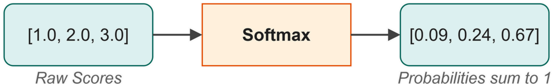
Figure 3.4: Softmax forces numbers into a 0-to-1 range where they total exactly 1.0.
